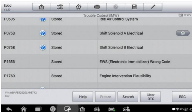
Figure 6-7 Sample DTC & FFD Screen
