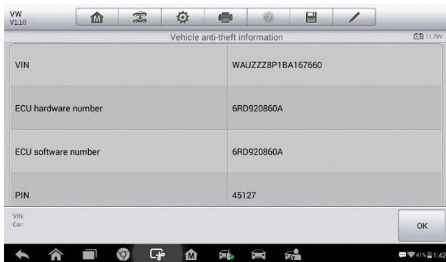
Figure 4-15 Sample Read IMMO Data Screen
