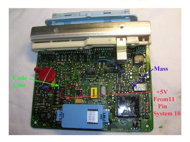
In the engine driver find a Motorola processor F1 and to use emulator in line FE10 type twice 73 00 73 00.
