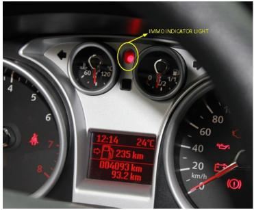
According to the instruction on screen, you should insert a new key and turn IGN on. You may see the IMMO indicator light will flash when inserting a key which cannot start Engine.
