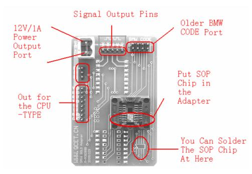
SOP IC in the socker with the clamp.
