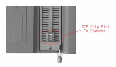
DIP IC in the socker without the clamp.
