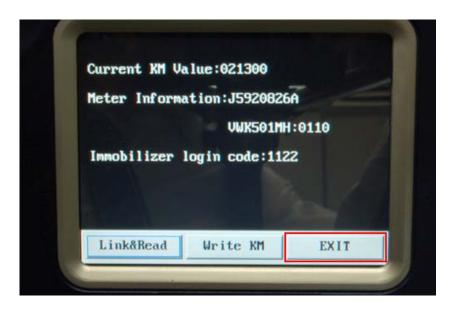
(12) Check if it displays the right mileage and disconnect the wiring.
