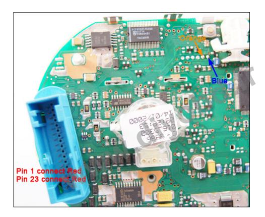
3. After that, pls connect the ICP and DIGIMASTER II body exactly:
