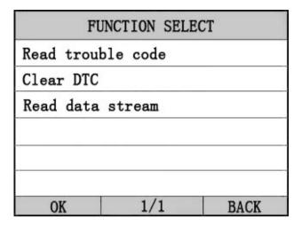
Press  $[\blacktriangle][\blacktriangledown]$  to select,  $[\blacktriangleleft]$  and  $[\blacktriangleright]$  to Page, and press  $[\longleftarrow]$  to confirm.
