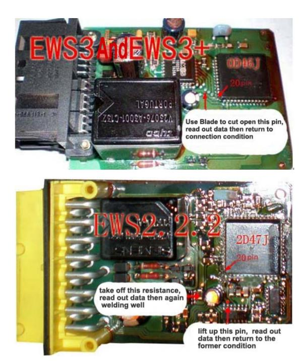
Then, handle well every pin of CPU, correctly put the IC socket
