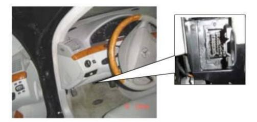
\*Benz S320,220 Chassis: the OBD plug is below the dashboard, use SMART OBDII-16 connector.
