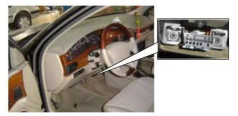
\*GM Buick: the OBD plug is below the dashboard, use SMART OBDII-16 connector.
