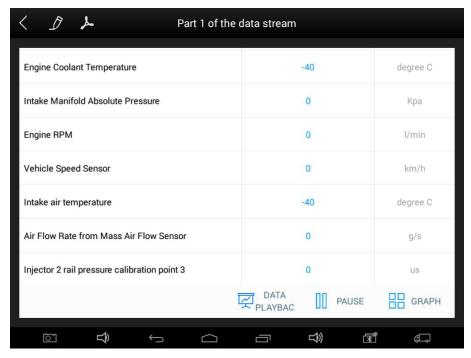
Tip: Live Data is important function that can be used to help technicians further diagnose a problem. This function requires technicians to be familiar with sensor data of each system, control signals and control modes. Tip: Save known good live data readings for comparison.
