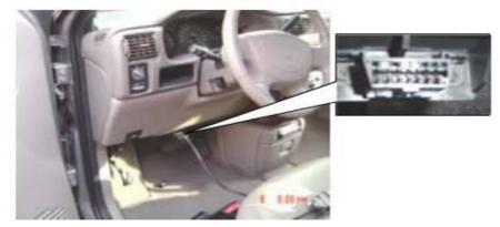
\*GM Buick GL8 : the OBD plug is below the dashboard, use SMART OBDII-16 connector.
