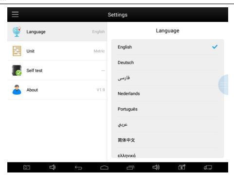
Units: Select unit of measurement. Users can select Metric or British Unit.
