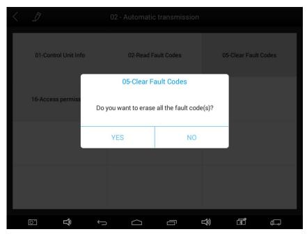
4.5.2. Click **YES** to confirm the operation, if the communication is normal, it will show "**Trouble Codes Successfully Cleared**" or "**Trouble Codes Cleared**". Generally, users will need to re-read trouble codes after clearing them to confirm that the trouble codes have been cleared.
