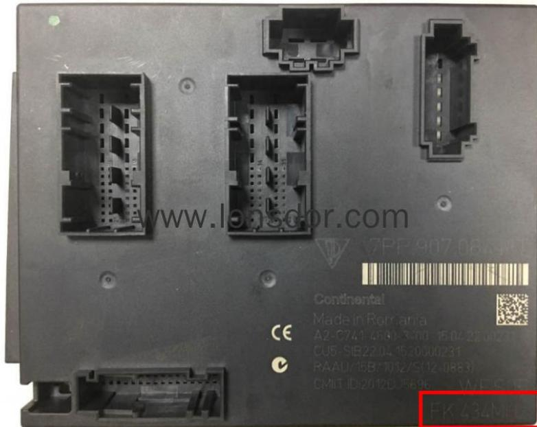
2. Read the BIN (D-FLASH / EEPROM) file with the programmer specifically for reading BCM. Please pay attention to the type here: namely 1L15Y 2M25J metal crystal, or 5M48H 1N35H ceramic crystal (red mark):
